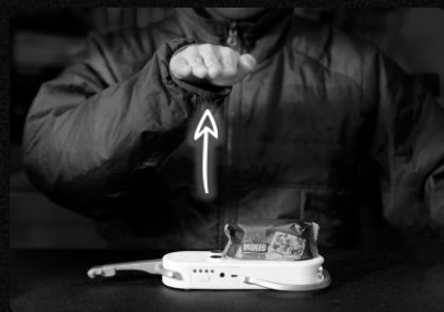
3. Raise and lower your right hand. Distance control pitch level (Each 2.4cm distance make one pitch change)
